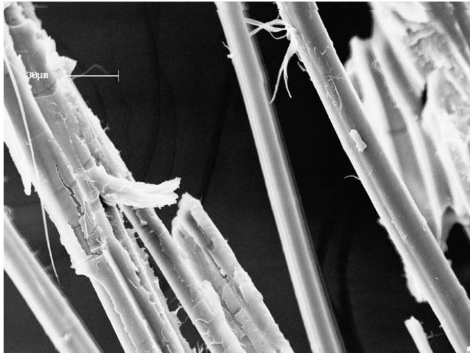
Figure 10 SEM photomicrograph of fibers just above the fractured surface of composite specimen with 15 mm fiber length and 30% fiber content.
